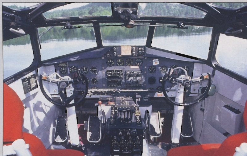
ABOVE A fine view of the flightdeck — and typical Sproat Lake scenery beyond. The Mars operates with four crew, and during firefighting the flight engineer handles the throttles.
